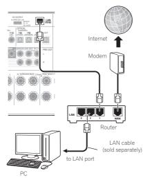
Connect the LAN terminal on this receiver to the LAN terminal on your router (with or without the built-in DHCP server function) with a straight LAN cable (CAT 5 or higher). Turn on the DHCP server function of your router. In case your router does not have the built-in DHCP server function, it is necessary to set up the network manually. For details, see *Network Setup menu* on page 68.
